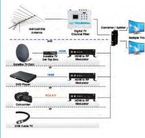
ST-8802 can work with HDMI to RF modulator to combine multiple HDMI video channels with Terrestrial or Cable TV channels
