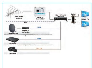
ST-8802 can replace several components in delivery path of TV signals, including channel (signal) booster, filter, frequency converter, combiner, equalizer and amplifier
